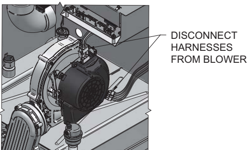
Figure 5-7 Disconnect harnesses from blower
